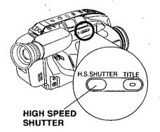
Press <u>HIGH SPEED SHUTTER</u> while recording.
